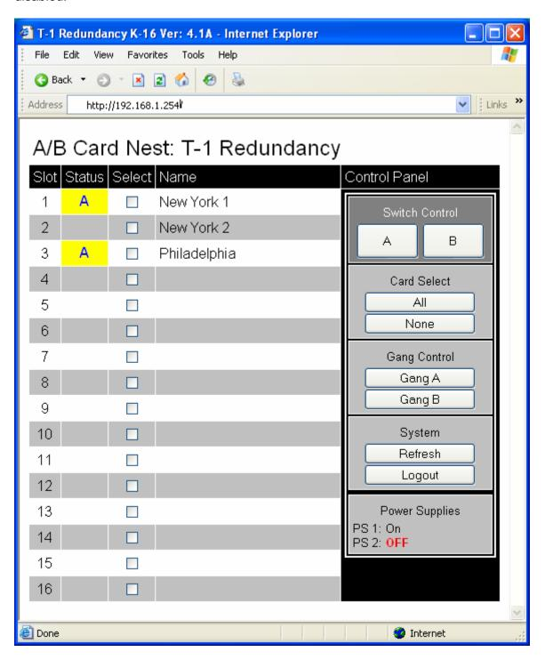
To simultaneously switch all cards in the chassis, click on either the Gang A or Gang B buttons. The checkboxes need not be used for this operation.
